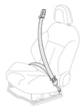
The front seat belts are fitted with a pretensioning and force limiting system. This system improves safety in the front seats in the event of a front or side impact. Depending on the severity of the impact, the pretensioning system instantly tightens the seat belts against the body of the occupants. The pretensioning seat belts are active when the ignition is on.
