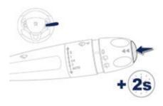
When the trip required is displayed, press the control for more than two seconds or use the left hand thumb wheel of the steering mounted controls.
