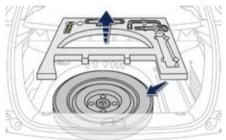
The spare wheel is installed in the boot under the floor.
