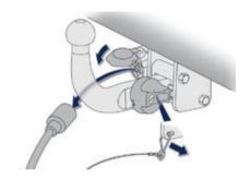
Disconnect the trailer harness from the socket on the carrier.
