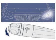
Side markers for the vehicle by illumination of the sidelamps on the traffic side only.
