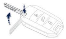
Press this button to unfold the key.
