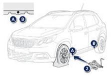
Place the foot of the jack 2 on the ground and ensure that it is directly below the front A or rear B jacking point provided on the underbody, whichever is closest to the wheel to be changed.
