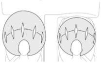
System which protects the driver and front passenger in the event of a serious front impact, in order to limit the risk of injury to the head and thorax.
