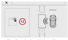
Move forwards alongside the parking space at a speed below 12 mph (20 km/h) to measure it, keeping at a distance of between 0.5 and 1.5 metres from the row of parked vehicles.
