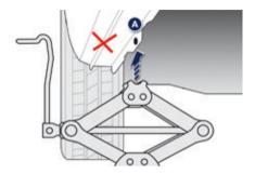
Raise the vehicle until there is sufficient space between the wheel and the ground to admit the spare (not punctured) wheel easily.
