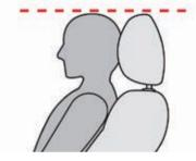
The head restraint has a frame with notches which prevent it from lowering; this is a safety device in case of impact. The adjustment is correct when the upper edge of the head restraint is level with the top of the head.
