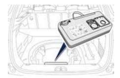
This kit is installed in the storage box, under the boot floor.
