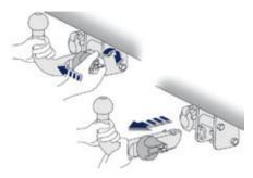
Grasp the towball firmly with one hand; with the other hand, press and turn the locking wheel clockwise as far as it will go.
