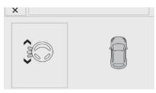
Operate the direction indicator on the parking side.
