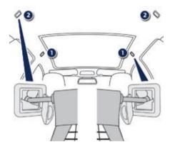
Hooked onto the upper fixings and onto the lower rings or the lugs, this permits use of the entire loading volume up to the roof:
