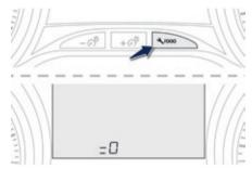
After each service, the service indicator must be reset to zero.
