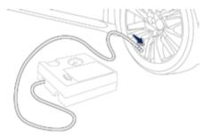
To check and if necessary adjust the tyre pressures.
