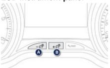
With the headlamps on, press button **B** to increase the brightness of the instruments and controls and the interior mood lighting or button **A** to reduce it.
