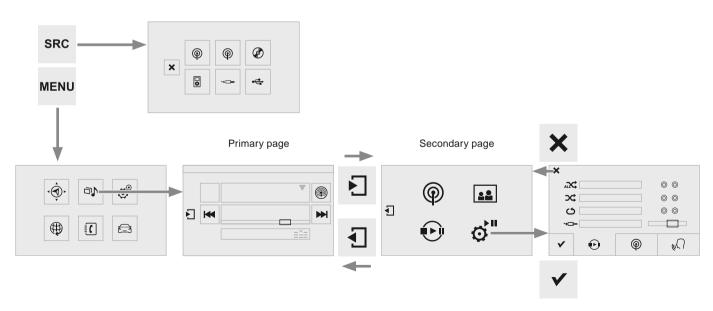
Short-cuts: using the touch buttons in the upper band of the touch screen, it is possible to go directly to the selection of audio source, the list of stations (or titles, depending on the source).
