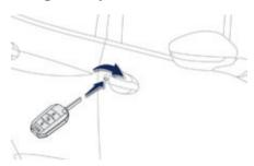
Turn the key in the driver's door lock towards the rear to lock the vehicle.
