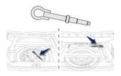
The towing eye is installed in the boot under the floor.
