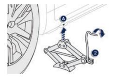
Extend the jack 2 until it comes into contact with the jacking point A or B used; the contact area A or B on the vehicle must be correctly inserted into the central part of the head of the jack.
