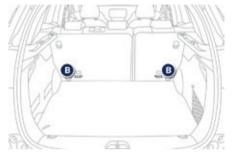
a ring B behind the seat for fixing the upper strap, referred to as the TOP TETHER.
