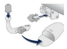
Refit the protective cover for the ball. Stow the towball in its bag. Refit the protective blanking plug to the carrier.
