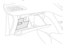
The extraction tweezer is fitted to the back of the fusebox cover located inside the glove box.
