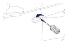
Insert the key in the lock to lock or unlock the door.
