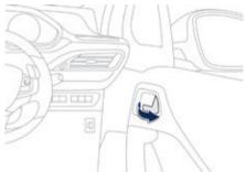
Pull the interior control lever of a front door; this unlocks the vehicle completely.
