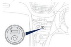
This connection box, consisting of an USB port and a JACK auxiliary socket is located on the centre console.
