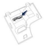
remove the carrier on which the tweezer is fitted.
