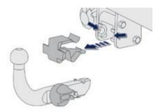
Remove the protective blanking plug from the carrier and check the condition of the fixing system. If necessary, clean the carrier with a brush or clean cloth.
