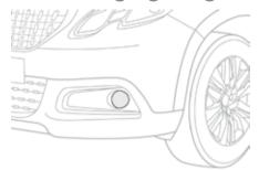
With dipped or main beams, this function makes use of the beam from a front foglamp to illuminate the inside of a bend, when the vehicle speed is below 25 mph (approximately 40 km/h) (urban driving, winding road, intersections, parking manoeuvres...).
