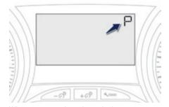
When you move the selector in the gate to select a position, the corresponding indicator is displayed in the instrument panel.
