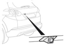
The reversing camera is activated automatically when reverse gear is engaged.
