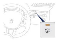
In the event of a fault with the system, the "ECO OFF" switch warning lamp flashes then comes on continuously.
