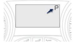
When you move the selector to select a position, the corresponding indicator is displayed in the instrument panel.
