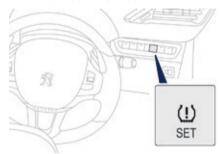
(!) SET With the ignition on and the vehicle stationary, press this button for about 3 seconds then release it, an audible signal confirms the reinitialisation.
