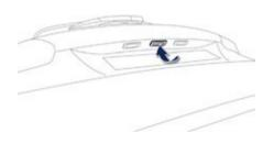
After unlocking the boot or the vehicle using the remote control or the key, press the opening control, then raise the tailgate.
