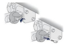
Check that the towball has correctly locked in place (position  ${\bf A}$ ).
