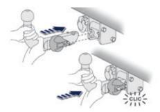
Take the towball in both hands; insert the end of the towball into the carrier, then, to ensure that it has correctly locked in place, pull firmly down on the ball end of the towball.
