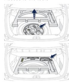
The tools are installed in the boot under the floor.
