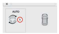
The assisted parking manoeuvre is in progress. Without exceeding 5 mph (8 km/h), continue the manoeuvres following the information given by the "parking assistance" system, until the end of manoeuvre message is displayed. The indicator lamp in the control goes off, accompanied by a audible signal.
