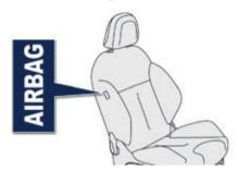
System which protects the driver and front passenger in the event of a serious side impact in order to limit the risk of injury to the chest, between the hip and the shoulder.
