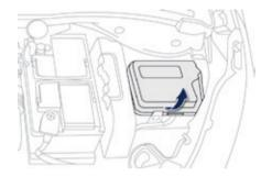
The fusebox is placed in the engine compartment near the battery (left-hand side).
