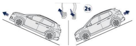
On an ascending slope, the vehicle is held for a brief moment when you release the brake pedal:
