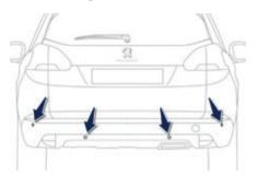
This system indicates the proximity of an obstacle (pedestrian, vehicle, tree, gate, etc.) which comes within the field of detection of sensors located in the bumper.
