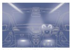
At night, interior mood light emitting diodes -LEDs (courtesy lamp, instrument panel, footwells, back-lit roof lining, panoramic glazed sunroof\*...) come on automatically when the sidelamps are switched on.
