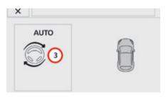
The assisted exit from parking manoeuvre is in progress.
