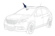
Using a laser sensor located at the top of the windscreen, this system detects a vehicle running in the same direction or stationary ahead of your vehicle.
