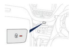
Press the button to lock (the indicator lamp in the button comes on) or unlock (the indicator lamp in the button goes off) the doors and boot from inside.
