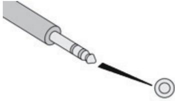
The auxiliary Jack socket permits the connection of a portable non-mass storage device or an Apple® player if not recognised by the USB port.
