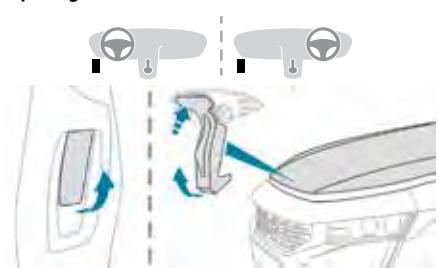
☞ **From inside:** pull the release lever, located on the left below the dashboard, towards you.
