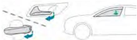
Your vehicle has doors with frameless windows. A window micro-descent system is activated when the door is opened and closed, as soon as an action is performed on its outer or inner door handle.
