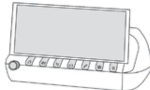
Use the buttons arranged below the touch screen for access to the menus, then press the virtual buttons in the touch screen.
