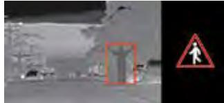
At night or in conditions of reduced visibility, the system uses an infrared camera at the front of the vehicle to identify and signal the presence of pedestrians and animals up to 200 m ahead of the vehicle, beyond the range of the main beam headlamps.
