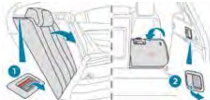
Each section of the backrest has two release controls:
